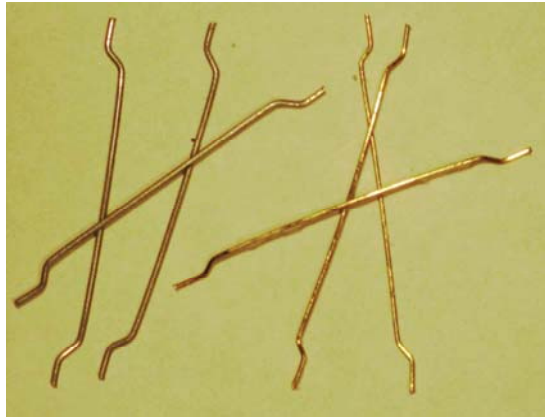
Fig. 4. Steel fibers used in this investigation (left: Specimen SB1; right: Specimen SB2)
